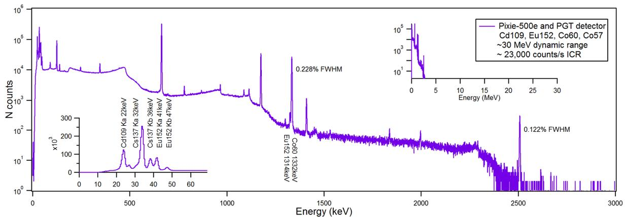
Fig.4: Even at fairly extreme conditions, ~30 MeV dynamic range and >20,000 counts/s, the Pixie-500e produces acceptable spectra. No artifacts due to nonlinearities are observed at low energy peaks, K $\alpha$  and K $\beta$  X-rays are well resolved, and resolutions are still ~0.12% at 2.5 MeV.
