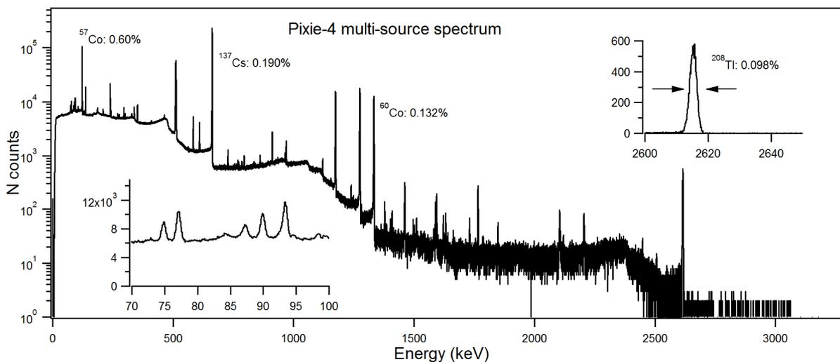
Fig. 2: Multi-source MCA spectrum for Pixie-4. The full dynamic range in this acquisition was about 3.6 MeV. Peak resolutions less than 0.1% FWHM can be achieved with a suitable detector, with no artifacts at low energy peaks.
