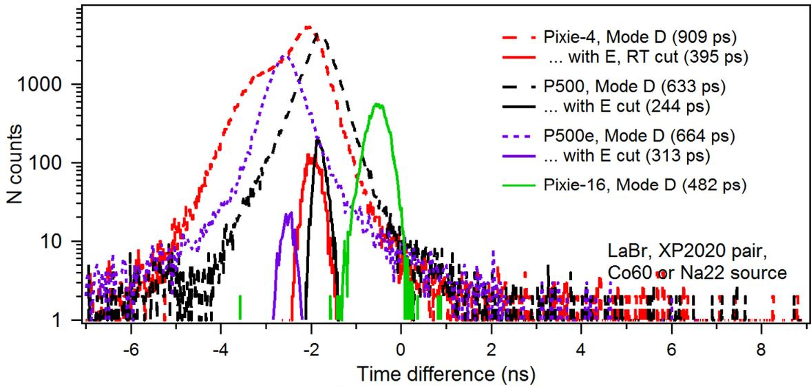
Fig. 8. Histograms of measured time difference  $\Delta T$  between two detectors with a coincident source (Na-22 or Co-60) fed into 2 channels (mode D). For the co-60 measurements, an energy (and rise time cut) can be applied to limit the analysis to pulses with  $E > 1\text{MeV}$ , which improves the timing resolution, but removes a significant number of events.
