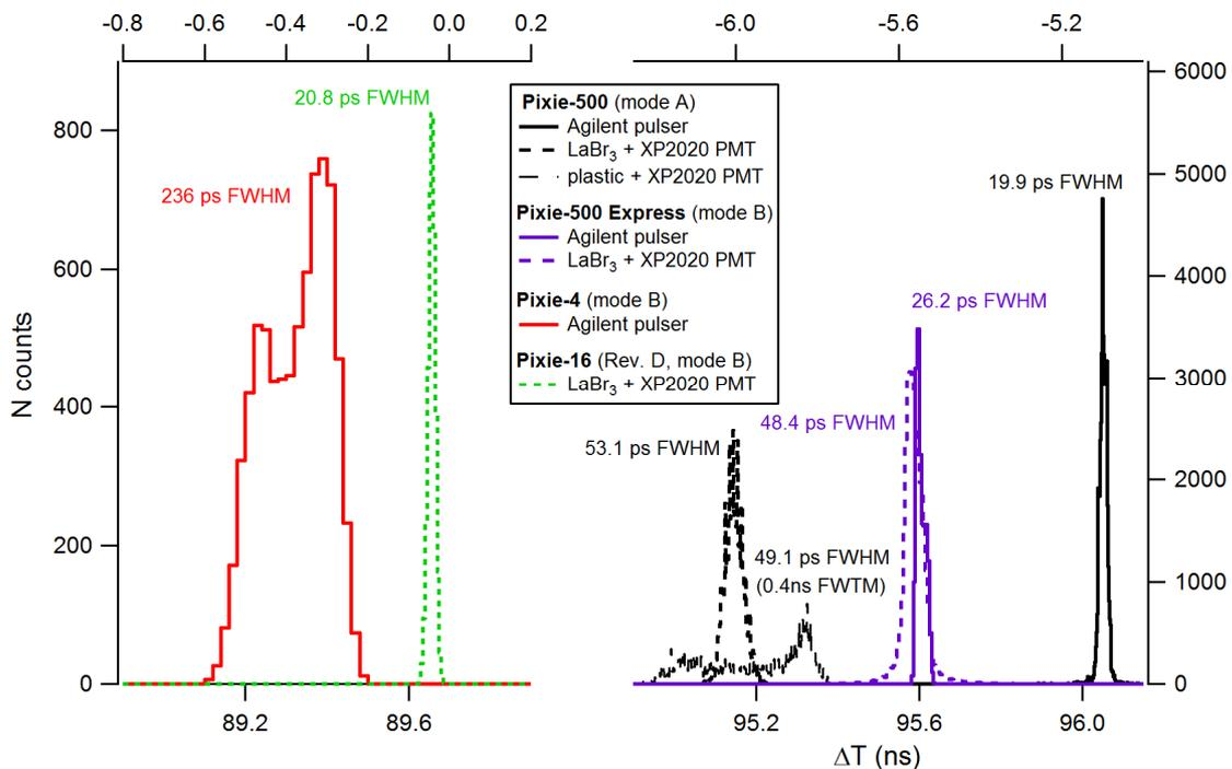
Fig. 7. Histograms of measured time difference  $\Delta T$  between the two rising edges of a double pulse (mode A) using P500, and between pulses split between 2 channels (mode B) using Pixie-4, Pixie-16 and Pixie-500 Express.
