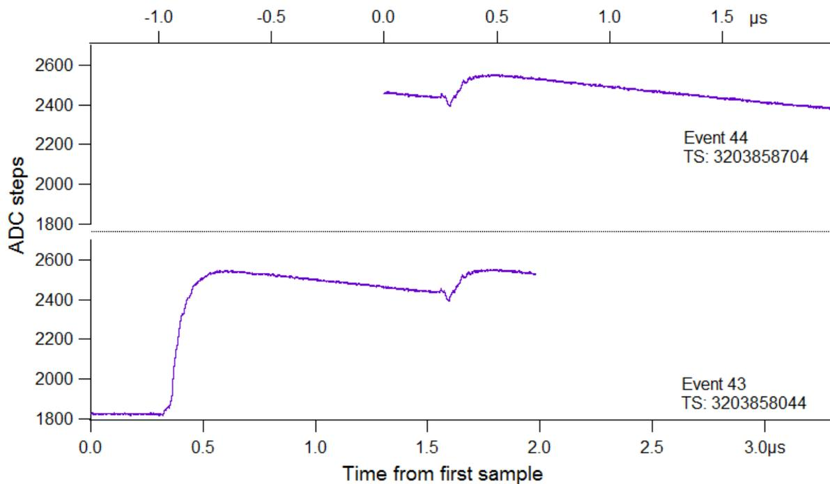
Fig.10: Capture of overlapping waveforms from closely following events with the Pixie-500e. The difference in time stamp TS is 660 clock cycles (1320 ns).
