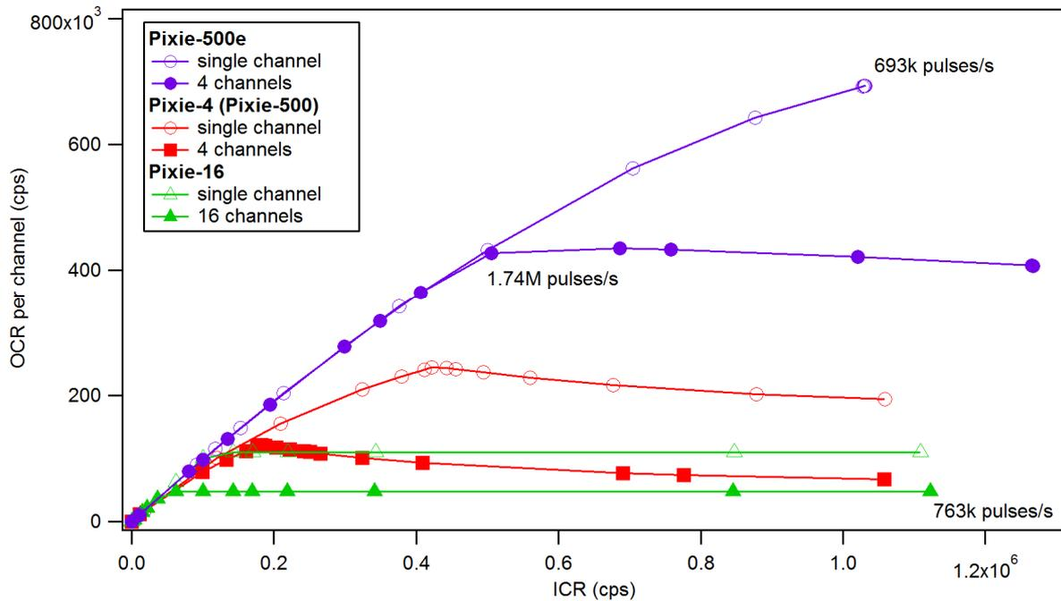
Fig. 5: Processed data rates (throughput of pulses *per channel*) for DGF Pixie modules. Measured in MCA mode with a random pulse generator with very short energy filter. Throughput as function of input count rate follows Poisson statistics until it reaches a plateau set by the processing limit (or decreases due to higher processing load).
