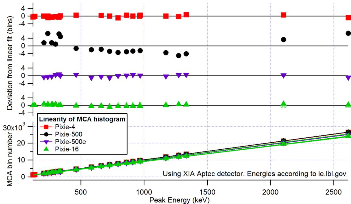
Fig. 7: Peak positions of multi-line spectra acquired with Pixie-4, Pixie-500, Pixie-500e and Pixie-16 as a function of nominal energy; as well as the deviation from a linear fit. Measured with XIA's Aptec detector with natural Th and Cs, Co and Na sources. The spectra were acquired for several hours at an input count rate of approximately 8kcps (Pixie-4, Pixie16) or  $\sim 1.2\text{kcp}$ s (Pixie-500, Pixie-500 Express).
