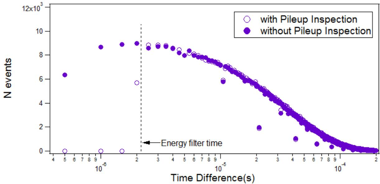
Fig.9: Histogram of time difference between subsequent events captured by the Pixie-500 Express. With pileup rejection enabled, the minimum time difference is the energy filter time. Without pileup rejection, the minimum approaches zero.
