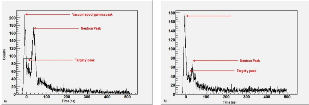
FIGURE 3. Detector counts in time a) Stilbene b) LaBr<sub>3</sub>
