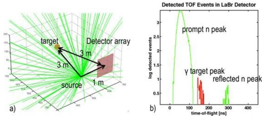
FIGURE 4. Monte Carlo Simulation a) geometric configuration b) Detector counts
