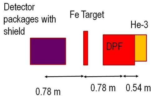
**FIGURE 1.** Experimental configuration to test Time-of-flight detection scheme.
