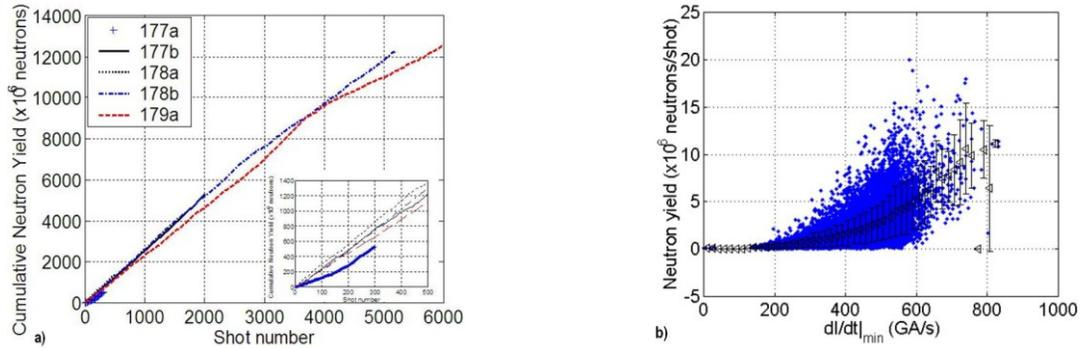
**FIGURE 2.** a) The cumulative neutron output over five different experiments. b) Neutron output vs. the minimum in the  $dI/dt$ .
