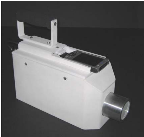
Figure 1. Photograph of the prototype CHELSI probe with 2"x2" CsI scintillator
